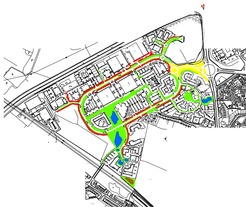
Figure 1: Plan of Aztec West development with retention ponds and detention basins. Drawing supplied courtesy of Peter Brett Associates.
